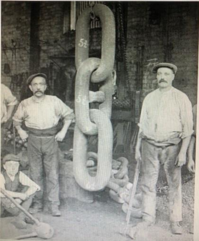
Making The Titanic's Anchor Chain At Hingley & Sons, 1909
